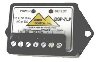
per second if the loop circuit is open and 10 times per second if the loop circuit is shorted. This detector operates in the fail safe mode and will output a "Detect" for either of these loop failure conditions. **This "Fail safe" detector should be used on "safety" loops.**
