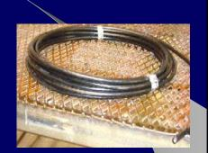
Cross-linked polyethylene has a melting point of 426°F
