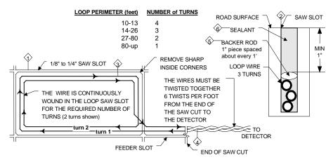
Recommended Loop Wire: Reno A & E LW-120 for 1/8-inch saw slots
