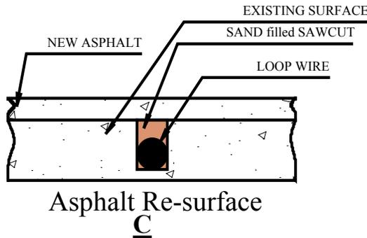
**Note:** Detection height is roughly 70% of the shortest side of loop.
